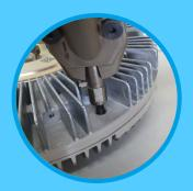
Our powerful pneumatic feed achieves a standard screw depth of up to 30 mm. Deeper screw points can be realized with the optional depth package. Additionally, the optional vacuum module is available. This can also be retrofitted at the factory for systems that have already been
