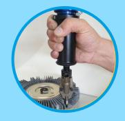
The TC-HF V2 features an ergonomic handle located directly behind the mouthpiece. This makes it easier to locate the screw point. The screwing process is initiated via the handle by slightly moving it in the screw direction. The mid-position stroke prevents the screw from sliding back into the mouthpiece. An optional lever
